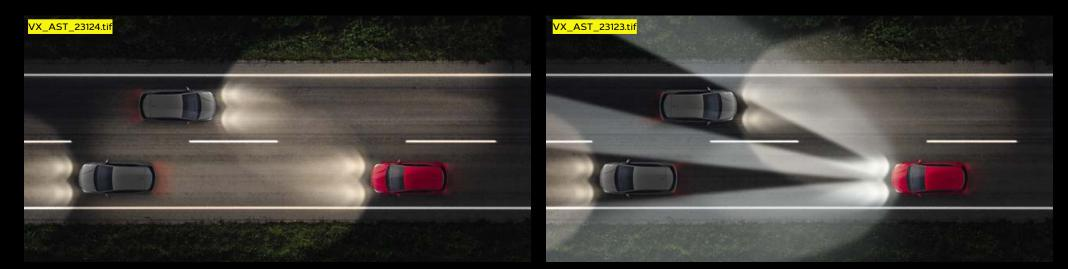
With standard halogen headlights, you have to switch between low and high beam to avoid dazzling drivers in oncoming cars.
