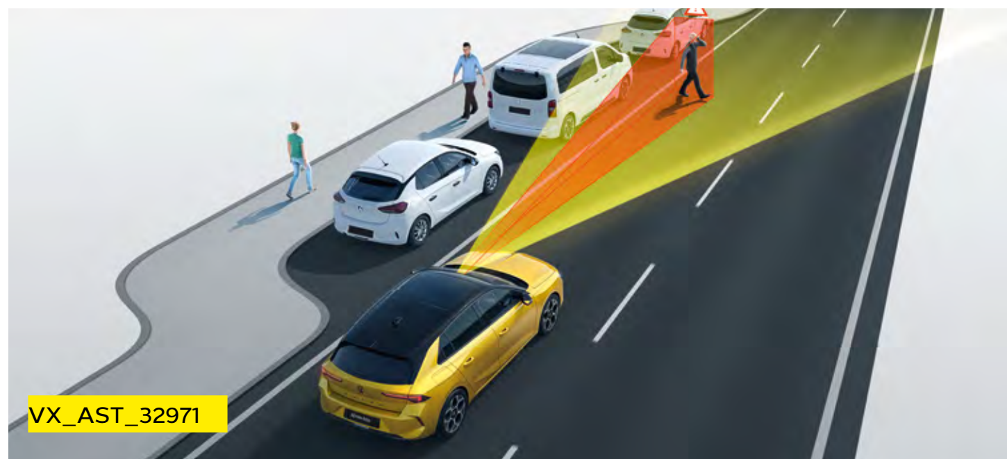
Automatic emergency braking with pedestrian protection.
