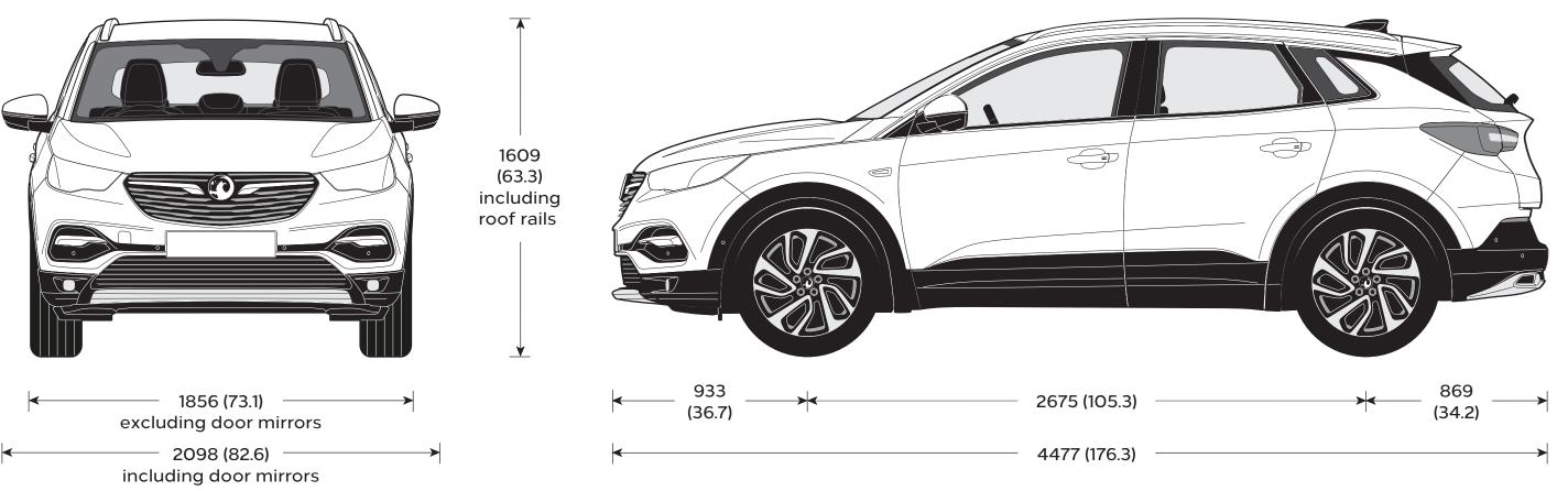
All measurements are in mm (inches) unless stated otherwise. \*Measured using the ECIE method.
