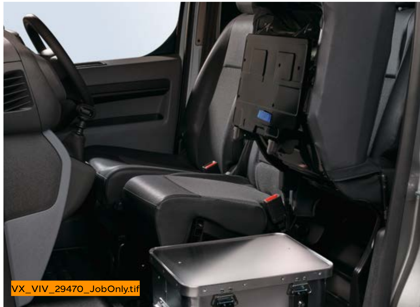
Load-through hatch within bulkhead.
