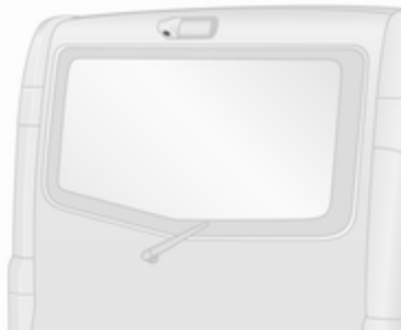
The camera is mounted above the rear doors / tailgate.
