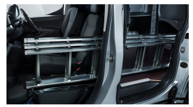
Load-through hatch within bulkhead.
