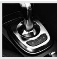
**Easytronic transmission** Choose any model with Easytronic transmission and you'll get a five speed manual gearbox with a fully automatic mode. In manual mode, you simply push the lever forward or back to shift gears up or down. The facia display tells you what gear you're in – 1 to 5. N for Neutral or A
