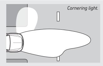
The 'Cornering light' uses an additional bulb and reflector to project a beam of light approximately 90° to the direction of travel when required – for example when turning at junctions or even negotiating tight roundabouts.
