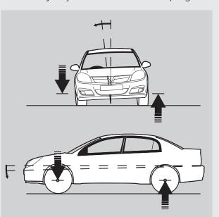
each wheel – effectively stiffening the suspension when required. This means that the vehicle will exhibit a reduced rate of roll and pitch, making it more responsive during direction changes and more settled during the braking/turn-in/acceleration transition when cornering.
