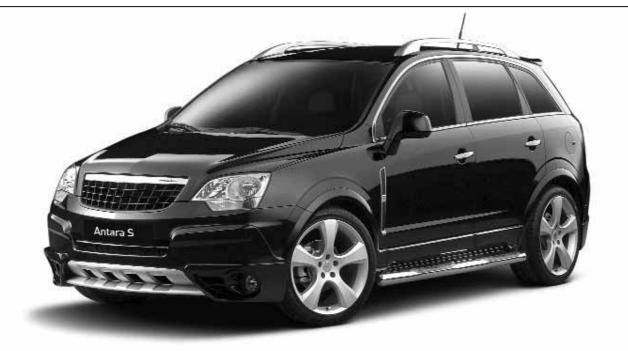
Antara illustrated features Irmscher front lower spoiler, cross hatch grille with aluminium upper, stainless steel door handle covers, side running boards, rear roof spoiler and 20-inch Evo Star alloy wheels.
