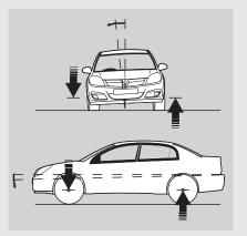
each wheel – effectively stiffening the suspension when required. This means that the vehicle will exhibit a reduced rate of roll and pitch, making it more responsive during direction changes and more settled during the braking/turn-in/acceleration transition when cornering.
