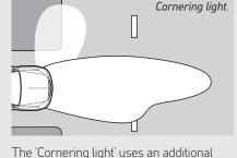
The 'Cornering light' uses an additional bulb and reflector to project a beam of light approximately 90° to the direction of travel when required – for example when turning at junctions or even negotiating tight roundabouts.
