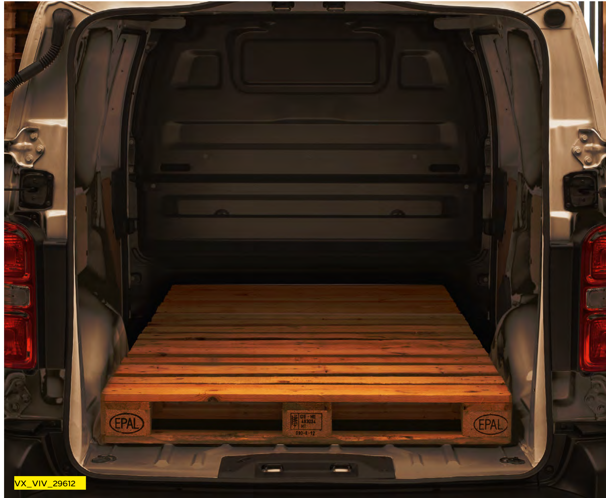
Full-height steel bulkhead.
